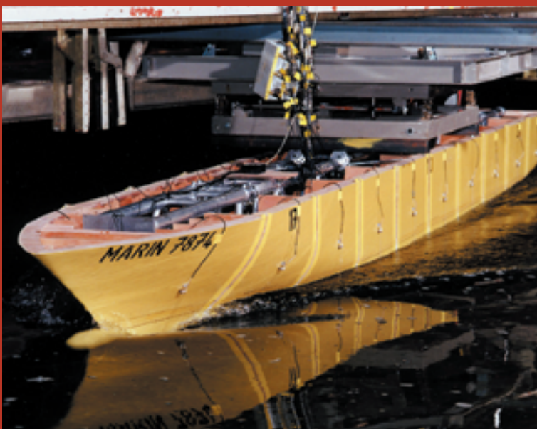
Manoeuvring tests on a segmented model.
